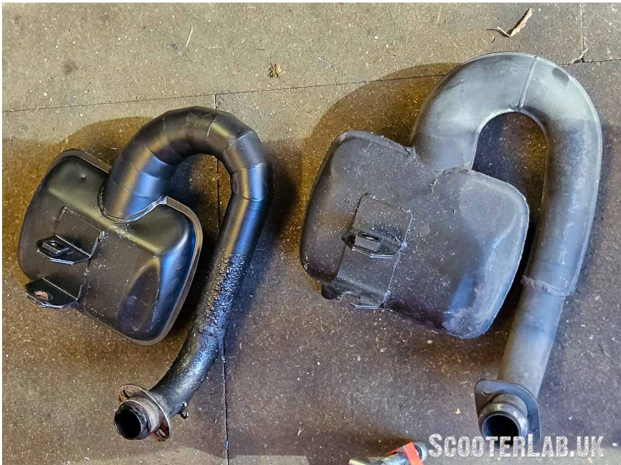
Modified White One Racing RPM exhaust with welded-on T5 stub (left) versus SIP Road 3 (right).
