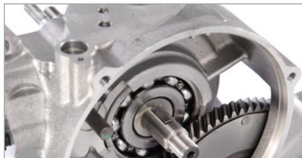
Clutch installation: put the woodruff key (part no 87070) in the groove. Make sure that it doesn't fly into the gearbox, groove pointing upwards! Then position the flat washer (part no 2229770) on the bearing with the bevel pointing downwards.
