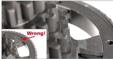
Ensure the correct installation of the primary gear cog, the edges have to be flush. The small image shows what it should not look like.
