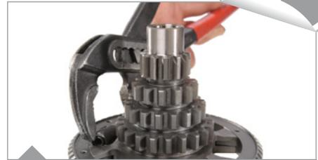
Insert the primary springs with the large set of pliers. Please note: on the Vespa PX200, two springs are intertwined.
