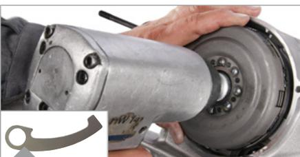
Tighten the clutch nut with the impact wrench (45Nm). Those who do not have an impact wrench are advised to use the clutch retaining tool (part no 909910).
