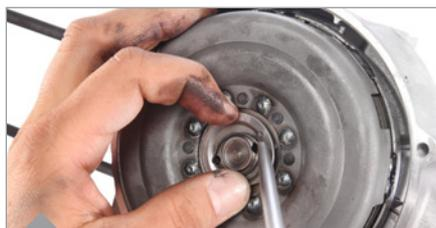
Fit the clutch pressure plate, firstly thread in the open spring ends then push down the spring with the flat screw driver until it snaps into position.
