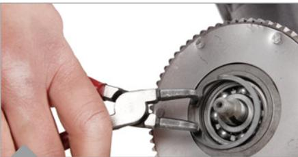
Put the input shaft in the gear cog set, bearings (put in freezer beforehand) with appropriate socket wrench insert (nut) tap in bearings until end stop. Secure with retaining circlip.
