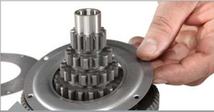
Waved cover disc to gear cog set, flat cover disc to clutch side. Fit rivets (head to flat disc). Fit the last rivet the other way around in order to start with the riveting work.
