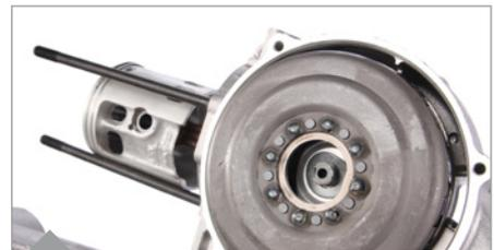
Push the clutch carefully over the woodruff key with the groove until it is positioned on the flat washer. Don't forget the wavy disc (part no 69820), then screw on the clutch nut.
