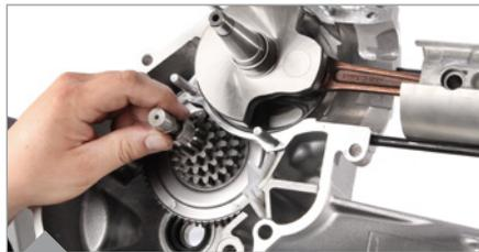
Thread the input shaft package into the engine case. Leave the input shaft sticking out a little to be able to insert the pins (part no 900810).
