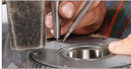
In order to rivet, put the input shaft on flat surface under vice. Attach the cover disc using the screwdriver. Tap in the first rivet using blunt driving hammer / hammer.
