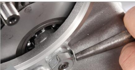
Screw in the input shaft with the lock washer, spacer washer and nut. Bend the lock washer on the nut with the driving hammer in order to secure it.
