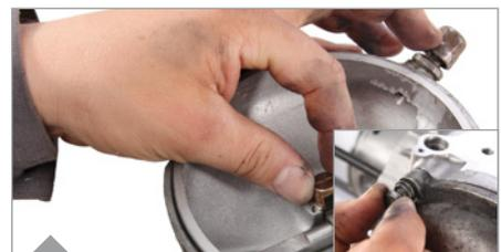
Put the O-ring (part no 92130) in the cover, insert the push rod (part no 87080), and attach the cover to the case with 3 screws.
