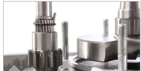
SIP Tip: thread in the pins apart from the last one and attach them with a suitable O-ring (from seal set, part no 92050). Pull the input shaft out a little and fit the last pin.
