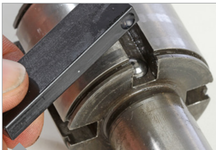
To fit the shifting ball bearings use tool part no 6379100. Do not forget new ball bearings (part no 637900) and reinforced springs (part no 1501150).
