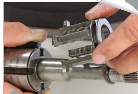
Fit the spring and both ball bearings to the drive shaft and fix them with both halves of the tool. Fit the new gear selector (e.g. part no 13490260), finished.
