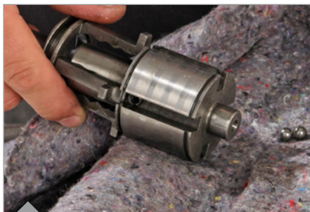
To disassemble the gear selector, knock the drive shaft into a cloth, pull the gear selector outwards and collect the shifting ball bearings on the left and right.
