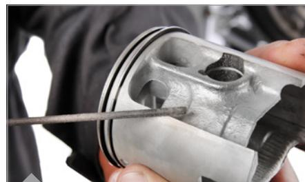
Make sure all edges and corners of the piston are chamfered and smoothed properly.
