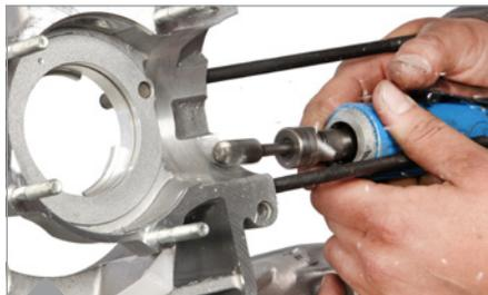
Remove the marked material using a drill or dremel with a suitable bit (e.g. PART NO 61626000)
