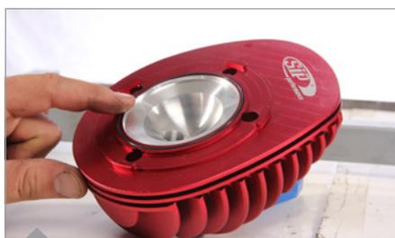
If you are using the SIP cylinder head apply the O-ring head gasket ...
