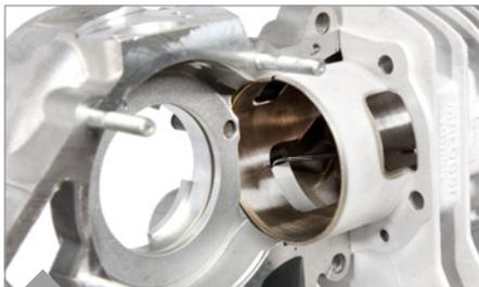
Push the cylinder onto the crankcase. Mark the shape of the transfer ports onto the base gasket surface w/ a scribe or marker pen.
