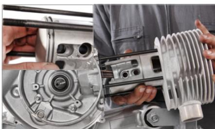
Mount base gasket. Oil the bore of the cylinder and push it gently over the piston. Ends of the rings should just touch the pins in the grooves.
