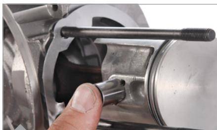
Install piston with the window facing upwards, install pin roller bearing. Push the gudgeon pin with a drop of oil into the piston
