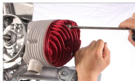
... and tighten the nuts crosswise to the same torque strength (between 17 and 21Nm) to suit.
