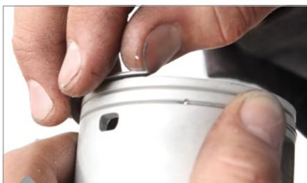
Install the piston rings carefully. This kit has wedge section rings, make sure the sloping surface faces towards the top of the piston.
