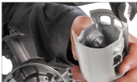
If you intend to use a 60mm stroke crankshaft the lower skirt of the piston should also be removed with a set of pliers or a file.
