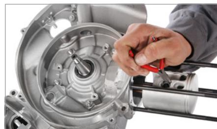
Put circlips into the grooves by using pliers. The POLINI 'G' circlips (# 13010000) also fit and are easier to install.
