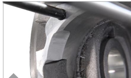
The depth/width of the transfers on the cylinder should be reproduced in the crankcase openings symmetrically, polishing is not necessary.
