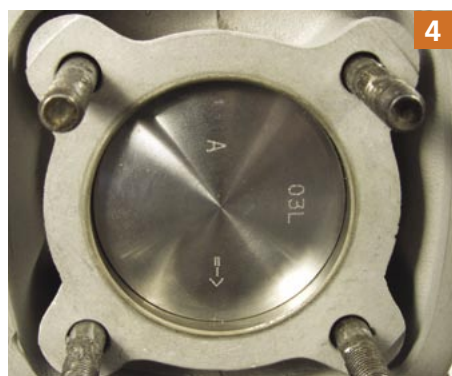
Pay attention which direction you place the piston. Arrow shows exhaust direction.
