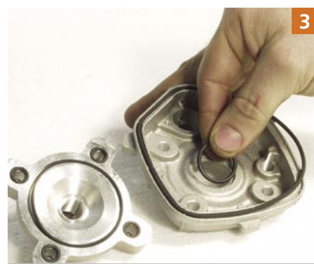
Always use new gaskets and o-rings. Always included in a new kit.
