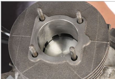
Here you see the original POLINI barrel while the piston is at the bottom of its stroke (BDC). The transfers haven't been completely uncovered.
