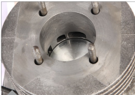
The raised POLINI at BDC, the transfer ports are completely open for improved port timings, a larger charge of fuel mix and higher rpm.
