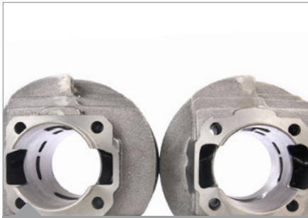
Through removing material from the base gasket surface area the transfer port have become noticeably larger and can supply a larger charge of fuel to the motor. Left: original POLINI Right: raised POLINI W5 version.
