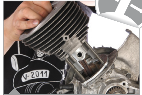
In order to mount the raised POLINI barrel the gasket spacer, also supplied with the kit, must also be included in the assembly.
