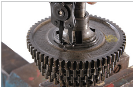
Open circlip (part no 151970). Remove gear cogs. Note the order! SIP-TIP: Tie together with cable ties.
