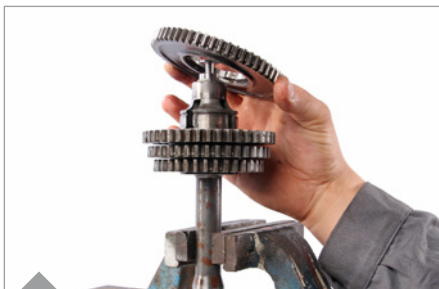
Put gear cogs in correct order on the main shaft. See mounting instructions at gear box technology chapter.
