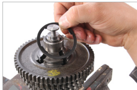
Insert spacer to compensate axial clearance. Recommended clearance 0.1-0.4mm. Use a feeler gauge part no 608240.
