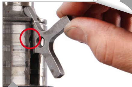
Thread the new cruciform. Attention, there's a cut-out at a groove on Lusso models to turn in the cruciform.
