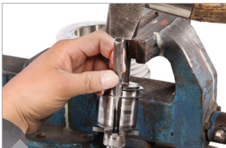
SIP-TIP: Punch mark the selector rod to avoid that the cruciform comes loose unintentionally.
