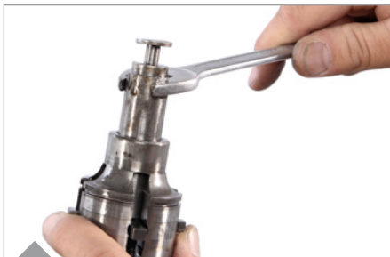
Unscrew the selector rod (left-hand thread!)
