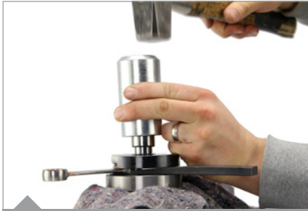
Use chuck part no 339710 to gently install the bearing.
