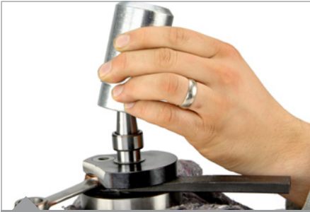
Position crankshaft on the bench vice and wedge the crankwebs with the Wedge crankshaft web part no 251270.
