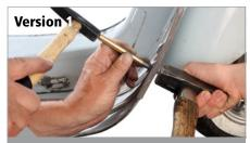
Attach the snap die (part no.131099) and hold the hammer against this. The rivet is jolted through targeted hits. Hold the snap die precisely 90° to the sheeting. An adhesive strip can also be applied to the bottom of the rivet in order to prevent scratches.
