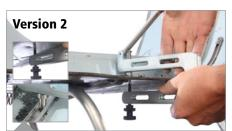
Apply the SIP riveting pliers (part no. 131040) with a smooth or semi-circular attachment. Screw down the opposite part in the form of the honeycomb pin and press the lever downwards to jolt the rivet. This makes riveting fun.
