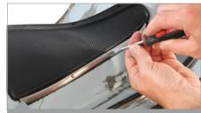
Where available, the floor mat floor board is affixed to the left and right using rails and 4 fillister head screws each.
