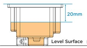
The fuel level should be ~20mm (.775 inches) down from the top of the float bowl flange while the float bowl is removed from the carburetor and resting on a flat, level surface.
